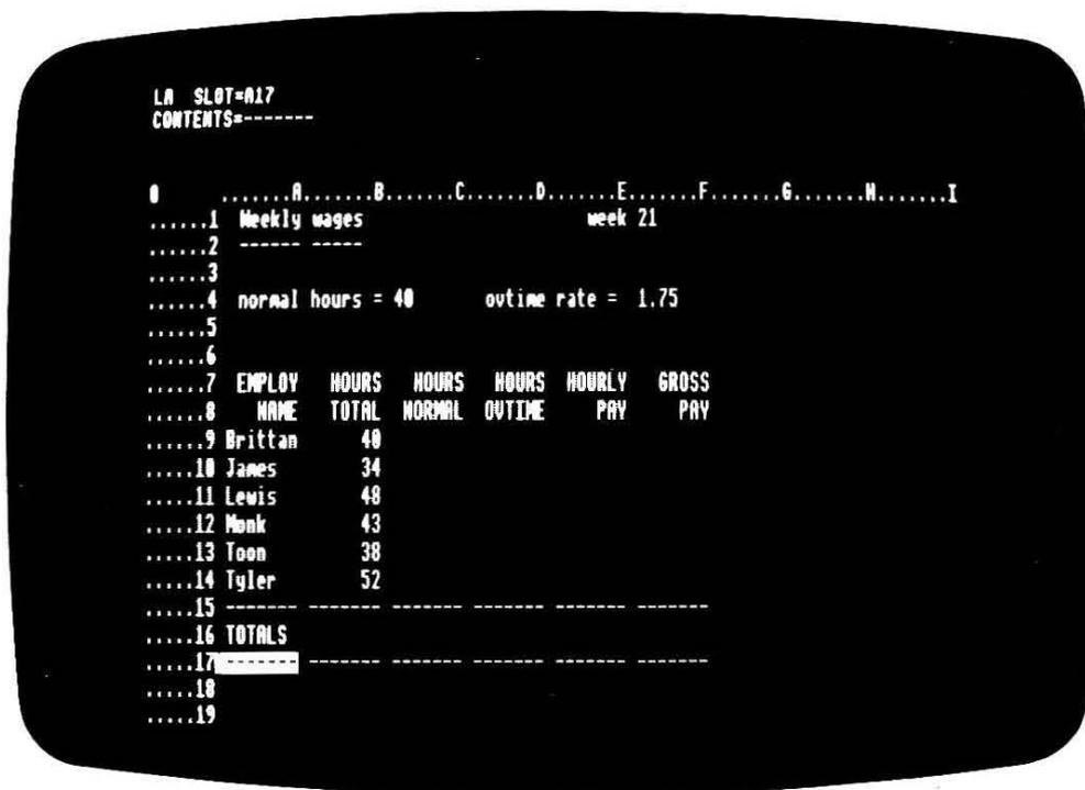
Before continuing, it is important to distinguish between values that must be entered directly, and those which ViewSheet can calculate from a formula. According to the rules outlined earlier, the HOURS NORMAL and HOURS OVTIME values can be calculated from the HOURS TOTAL. Similarly, the GROSS PAY will be calculated from values in the preceding columns. Therefore the only remaining values to be entered directly are those in column E, HOURLY PAY.
