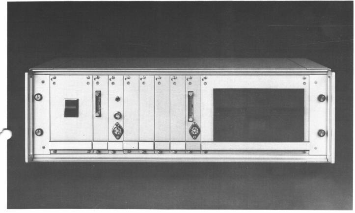
The System 3 Computer in its basic form is a system driving a single disk. The hardware consists of card frame, backplane with 4 sockets, 6502 CPU, VDU interface, 8K RAM, floppy disk module, DOS and resident 4K ASIC.
