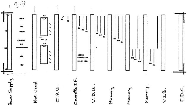
The cassette interface, VIB and the two empty locations may all be used for memory giving a 40K byte of RAM system. When fitting the buffers 9 wire links and a decoupling capacitor are also required on the front of the backplane.
