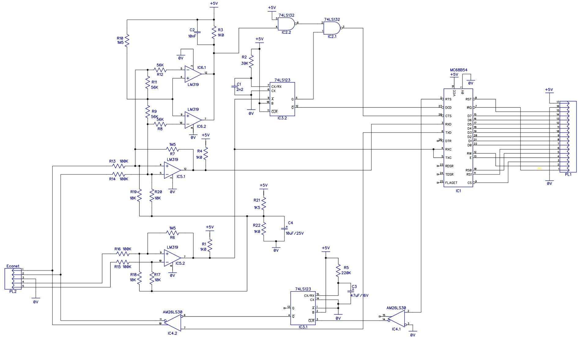
On the original the unused IC2 gate inputs were left floating
