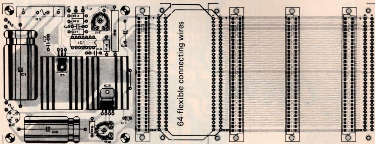
Figure 4. This figure illustrates the connections between the bus- and power supply boards.
