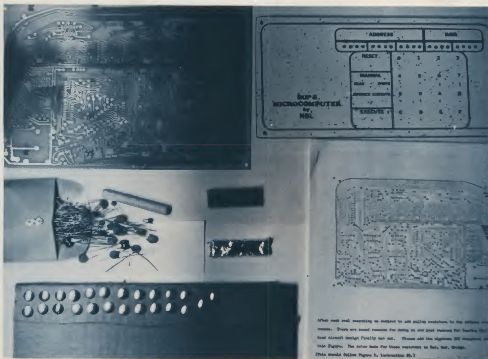
The SKIP II kit as it arrived in the mail. The black object in the center is the 40-pin socket for the SC/MP-II microprocessor chip, shown wrapped in foil just below the socket.
