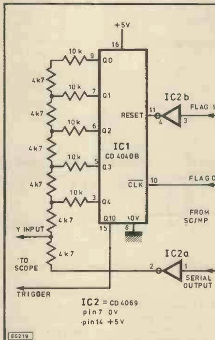
Fig. 1. Circuit for memory-mapped oscilloscope display
