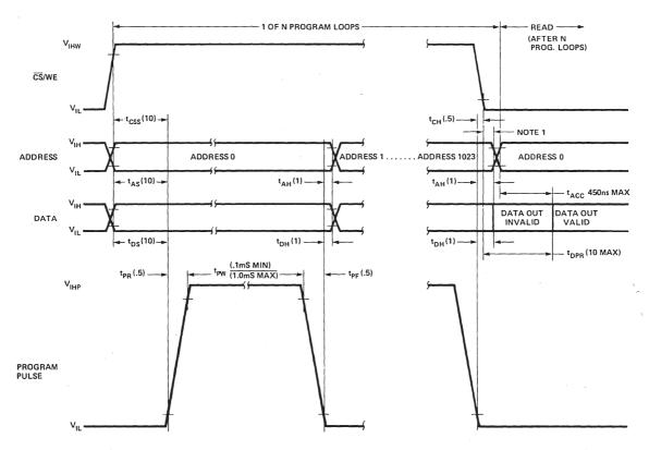
NOTE 1. THE  $\overline{\text{CS}}\textsc{Me}$  transition must occur after the program pulse transition and before the address transition.
